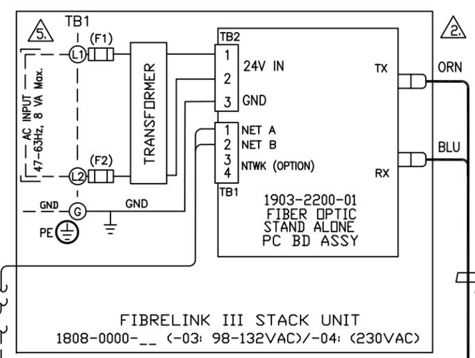
TWIN FIBER OPTIC CABLE REQ'D (62.5/125) WITH 'ST' TYPE CONNECTORS (4 FIBER RECOMMENDED) (LENGTH TBD PER SITE DATA)
