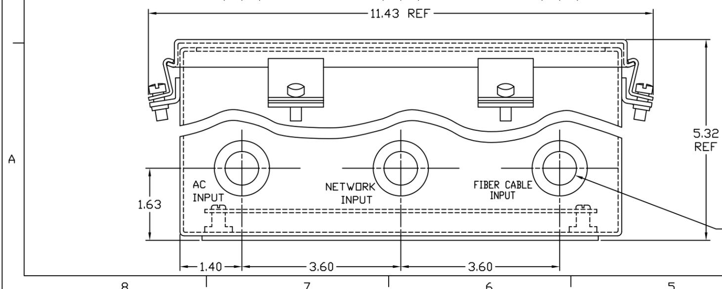
1/2" FLEX CONDUIT FITTINGS SUPPLIED BY MLI, FLEX CONDUIT SUPPLIED BY CUSTOMER. 3 PLACES
