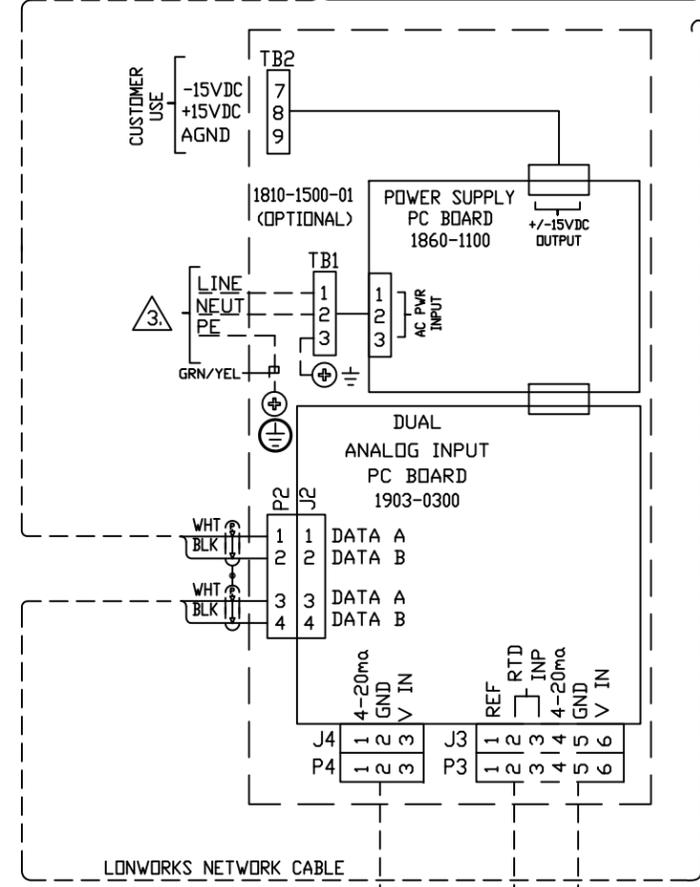
OPTIONAL WIRING FOR DUAL ANALOG INPUT MODULE
