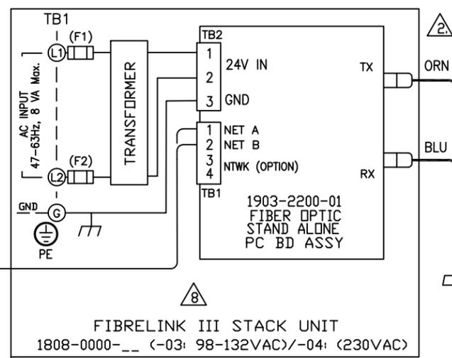
TWIN FIBER OPTIC CABLE REQ'D (62.5/125) WITH 'ST' TYPE CONNECTORS (4 FIBER RECOMMENDED) (LENGTH TBD PER SITE DATA)
