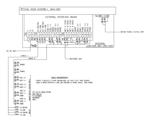
6PT I/O WIRING DIAGRAM
