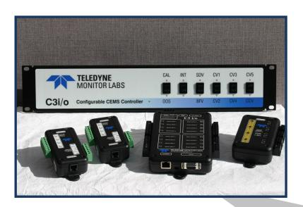
C3i/o, Configurable CEMS Controller with inputs and outputs, is designed to support and control one Continuous Emissions Monitoring System (CEMS) using a low cost, fully featured platform that's simple to configure and easy to operate. The CEMS can be a dilution system, an extractive system or a hybrid combination of both.
